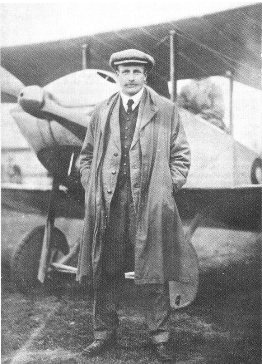
Fine man, fine aeroplane: Victor Mahl with a Tabloid having the 'racing', or V-type landing gear, fabric-faired wheels and one of several forms of engine cowling tried on the Tabloid. A spinner adds an extra sporting touch.
